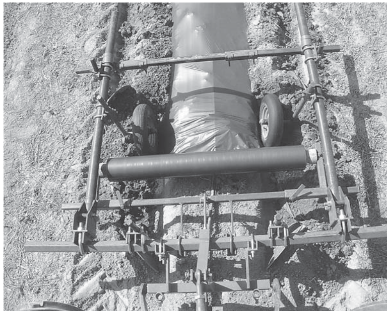
~ Photo 3 ~ Top view of thermal plastic mulch layer mounted behind tractor
