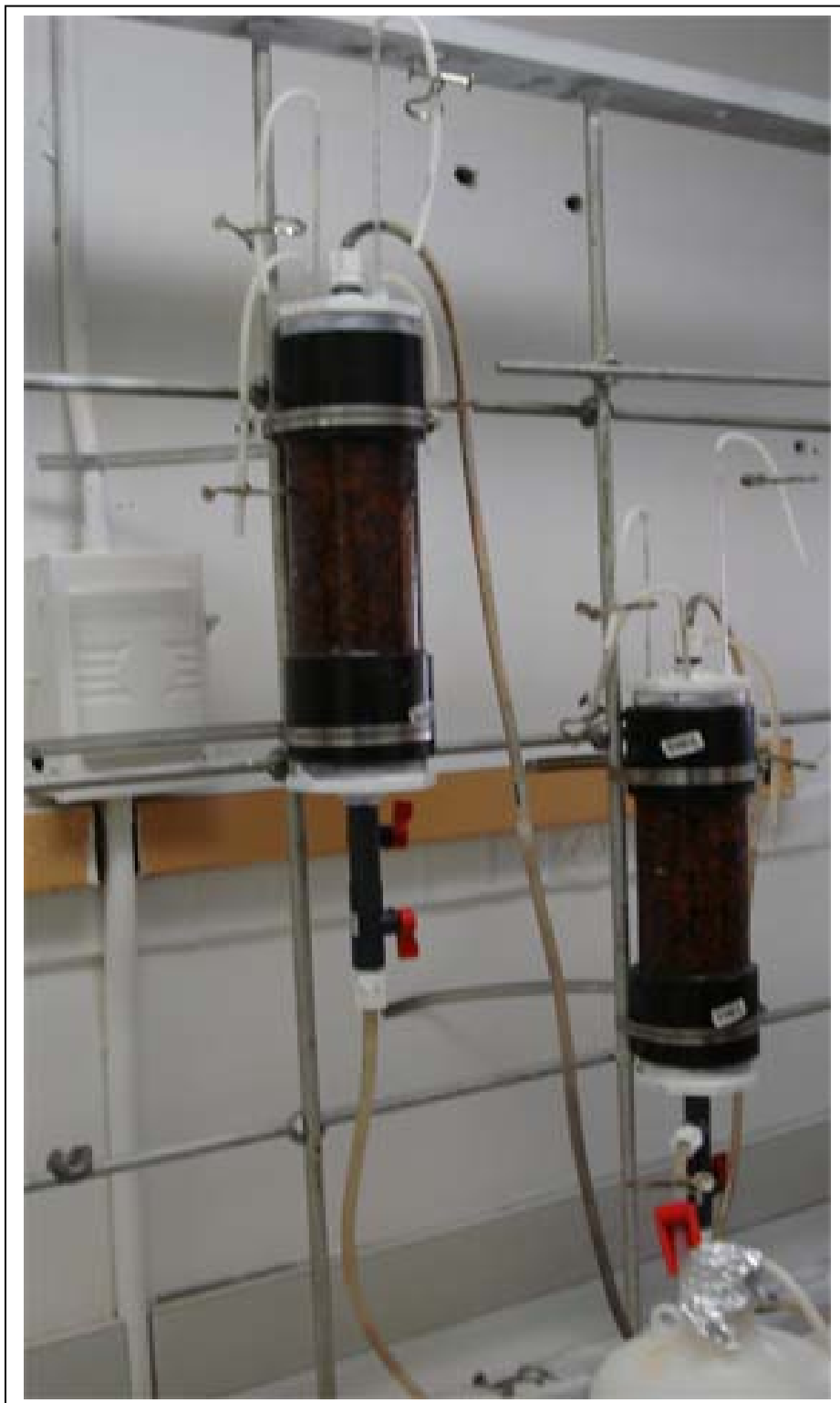
Figure 6. Two BEMR in series using a retention time of twenty-two hour each for a total retention time of forty-four hours.
