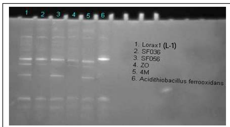
Figure 5. DGGE profiles of site microbial RNA from L-1 and ZO, two repository microbes, 4M - a mixture of all bioreactor test microbes, and a A. ferrooxidans control.
